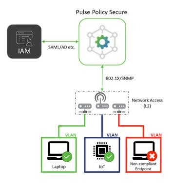
Figure 2: Dynamic access control and network segmentation (L2)
