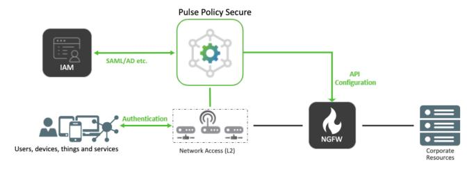
Figure 3: Dynamic access control at perimeter (L3)
